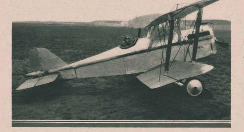
This is what might be called a "sky pen." It is used in spelling ont words in a white chemical smoke 10,000 feet in the air. The ezhanst pipe through which the smoke passes can be seen running along the side of the faselage
